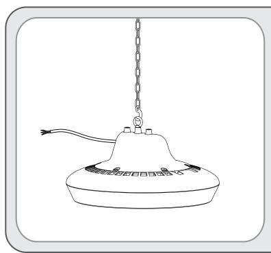
• Hoist the fixture up to the desired height and position by safely latching a hook through the O-ring provided on top of the fixture.
