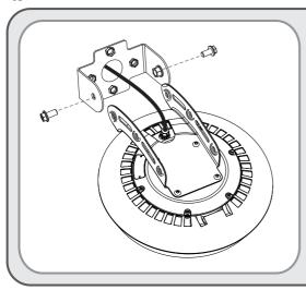
• After tightening the SWL Swivel Mount Bracket onto the intended surface firmly, align the light fixture bracket holes with the SWL Swivel Mount Bracket holes and tighten the fixture firmly at the desired angle.
