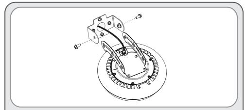
• For extended arm Swivel Mount system again align the light fixture Bracket holes with the extended arm Swivel Mount Bracket holes and tighten it firmly to the desired angle.
