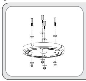
· Align and tighten the SST (Spring Loaded Snap and Turn Surface Mounting Bracket) onto the hexagon spacers using the hexagon nuts and washers provided in the kit.
