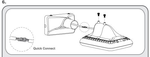
Connect the fixture to the AC input extension cable via the quick connector provided in the fixture kit.
