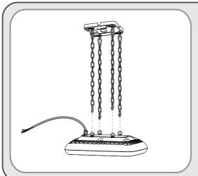
• Hang the fixture from the four chains by inserting the spring loaded hooks through the round eyelet anchors located on top of the fixture.
