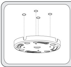
· Use the SST mounting bracket as a template to mark the screw holes location onto the intended surface.
