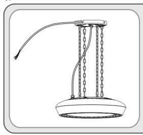
· Insert the fixture input AC cable wire through the center hole of the CH4 mounting bracket and pass it through the side exiting hole of the mounting bracket.
