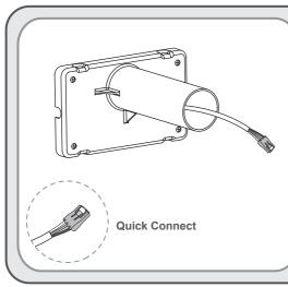
• Connect the AC input extension cable wire to power at the junction-box.
