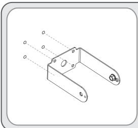
• Use the SWL Swivel Mounting Bracket as a template to mark the screw holes location onto the intended surface.
