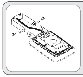
• After tightening the SWL Swivel Mount Bracket onto the intended surface firmly, align the light fixture bracket holes with the SWL Swivel Mount Bracket holes and tighten the fixture at the desired angle then tighten the two lock screws firmly to prevent any movement.
