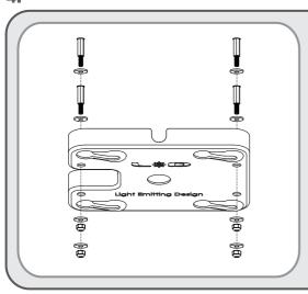
Align and tighten the SSL (Spring Loaded Snap and Slide Surface Mounting Bracket) onto the hexagon spacers using the hexagon nuts and washers provided in the kit.
