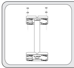
• Use the SSL mounting bracket as a template to mark the screw holes location onto the intended surface.
