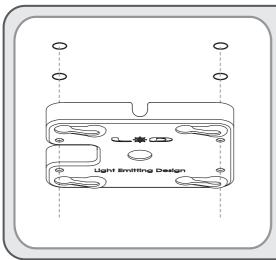
• Use the CH4 mounting bracket as a template to mark the screw holes location onto the intended surface.
