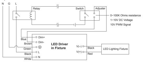
Using a switch and relay can turn ON/OFF the lighting fixture.
